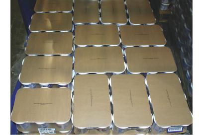
The grippers pull the pads from a stack and position them on the bottom and on top of stacked containers, above.
