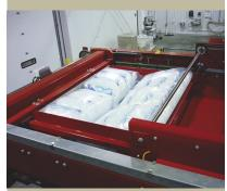
The palletizer's accumulation area is made of metal plates, which buckle up to move the ice to the stack below.
