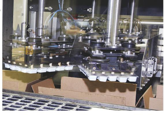
MULLINS FOOD PRODUCTS, a contract producer of condiments, uses a high-speed servodriven case packer to increase production speed, quality, efficiency and overall productivity.
