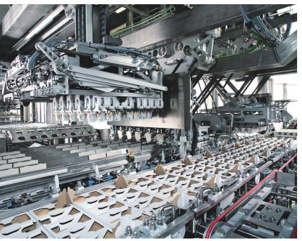
Sterzing's new yogurt cup-feeding/tray-packing system includes an array of stations that unitize cups transported directly from the new aspetic filler/sealer.
