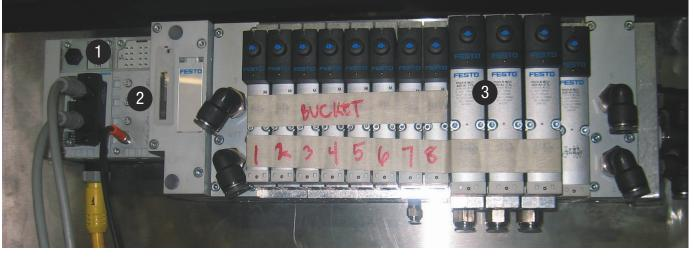
Controls for the rotary actuators on the trays that deliver product from the scale to the trays include (1) a DeviceNet node, (2) input module and (3) valves that open and close the rotary actuators on the
