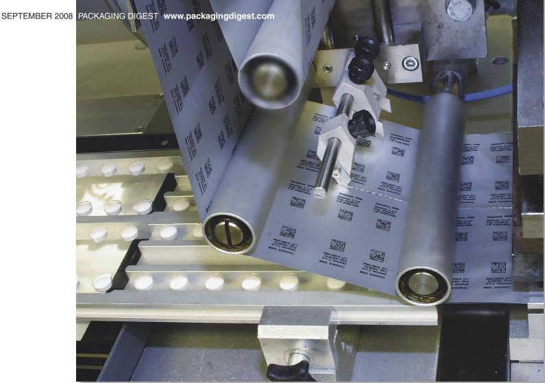
A filling machine places individual pills into a pouch and then seals them into a blister-pack. Tjoapack's packaging line prints a unique code for each pill in the package that can be used to identify and track it all the way through the supply chain to the final consumer.
