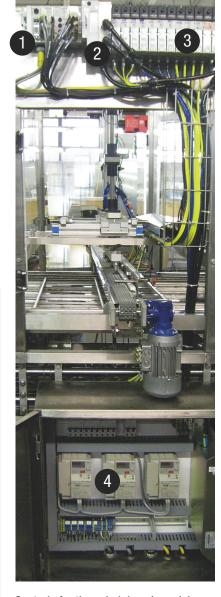
Controls for the salad dressing pickand-place unit, above, include a (1) DeviceNet node and I/O modules, (2) an air supply manifold, (3) solenoid valves for the vacuum cups and (4) variablespeed motor controls. The filler/sealer, below, includes 3 weighing systems. Product from each weighing system is delivered through 8 buckets arranged in 3 vertical levels to fill 4 trays at each machine cycle.
