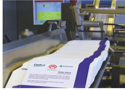
Once filled with blister-strips, medicine cartons have a 2D code imprinted, and the software aggregates that data with all the individual codes for tablets inside the carton.
