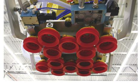
Suction cups are attached to the VGS 3010 gripper pickup heads. There can be 3 or 4 different pickup heads on 1 system.
