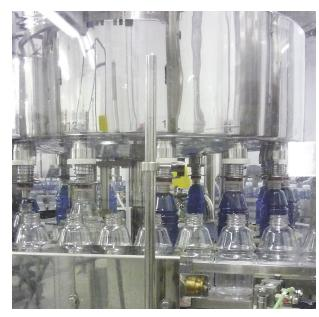
A 15-head filler, above, dispenses pasteurized and still hot grape Kwikade into 32-oz PET bottles. Air knives, right, blow water off bottles as they exit the cooling tunnel.
