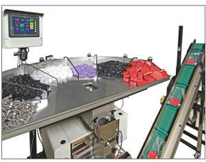
completed kits feed automatically into a film bag that gets sealed. A bar-code reader allows for instant job recalls, saves or queries. The US-5500 can be combined with the T-1000 Advanced Poly-Bagger™ and the Ti-1000 thermaltransfer printer.
