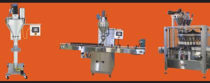
Inline Auger Fillers for manual to low speed applications
